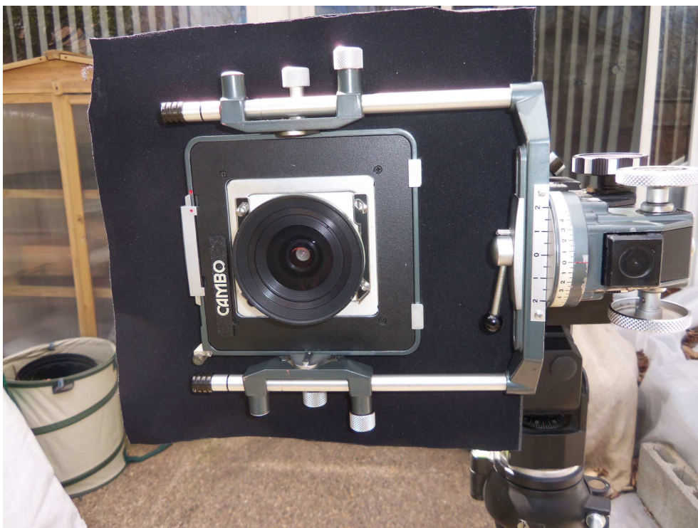
Figure 4: The bellows nearly completely compressed, 35 at infinity
