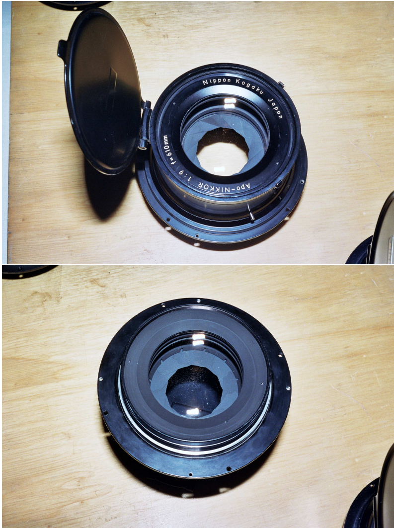
Figure 3: Symmetrical Apo Nikkor lens, dialyte type, focal length 610 mm
