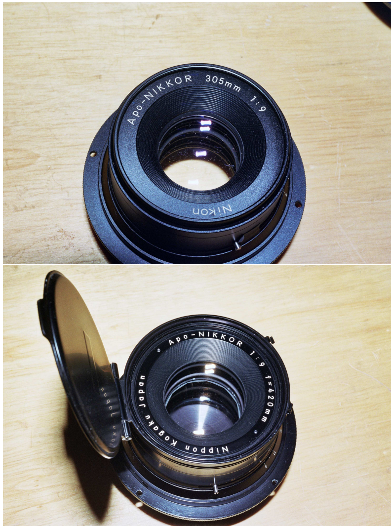
Figure 1: Symmetrical Apo Nikkor lenses, dialyte type, focal lengths 305 and 420 mm
