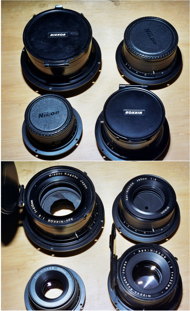
Figure 4: Four Symmetrical Apo Nikkor lenses, dialyte type
