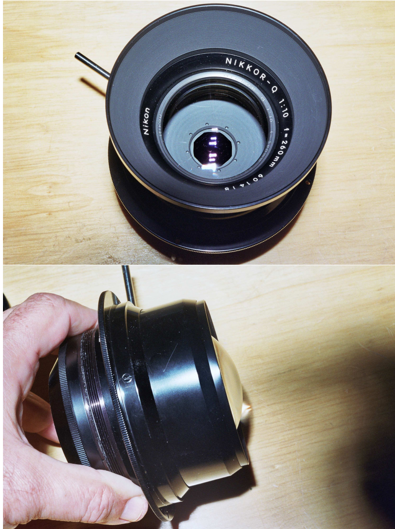
Figure 6: Nikkor-Q lens, double-Gauss type, focal length 260 mm; note the protruding rear lens element of this particular design.
