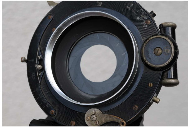
Figure 7: An example of iris diaphragm in an old Compound leaf shutter
