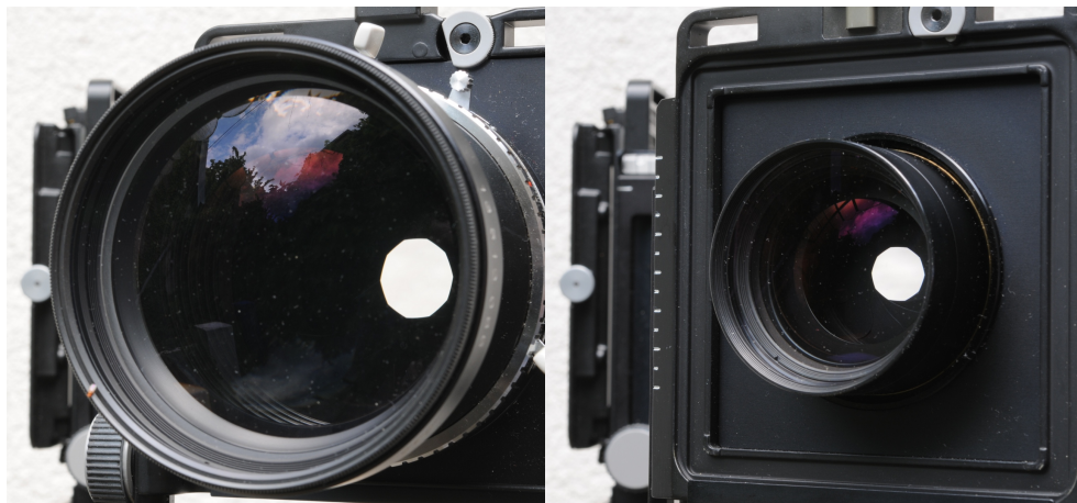
Figure 20: Entrance and exit pupil for the Schneider-Kreuznach Tele-Arton 360 mm lens. In this type of lens, the exit pupil has a smaller diameter than the entrance pupil, the pupil magnification (52) M_p is less than 1.
