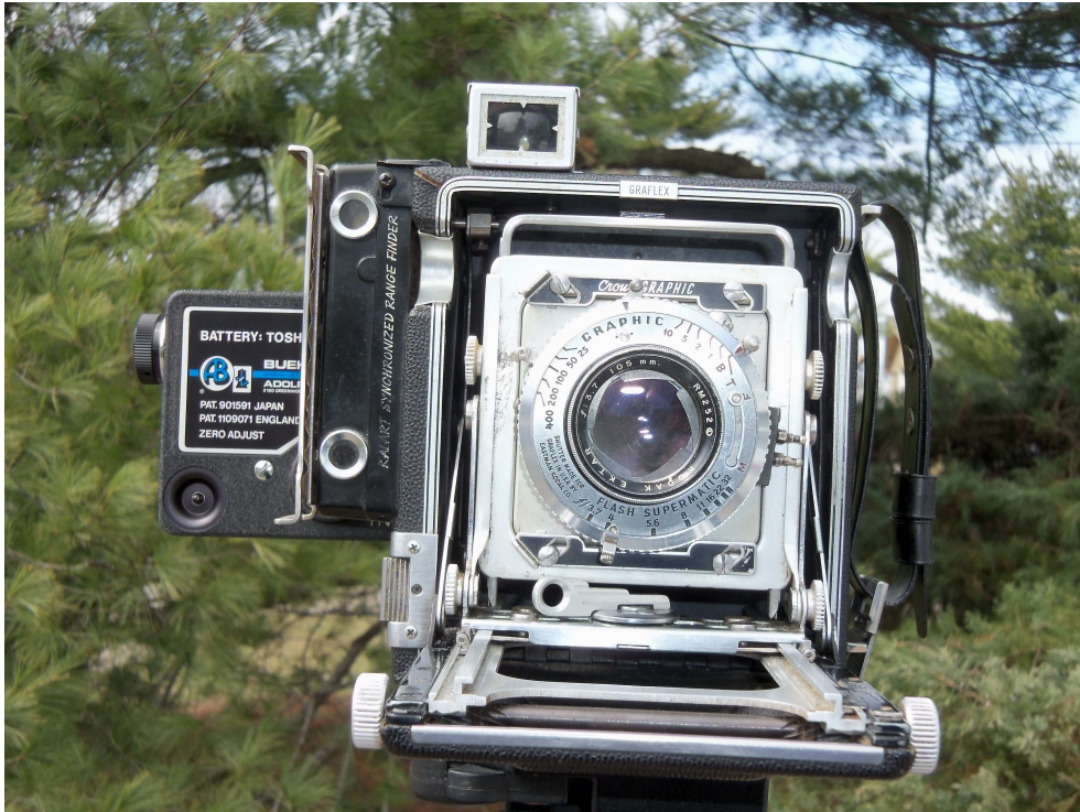
Figure 4: Meter in 2x3 Crown Graphic, front view
