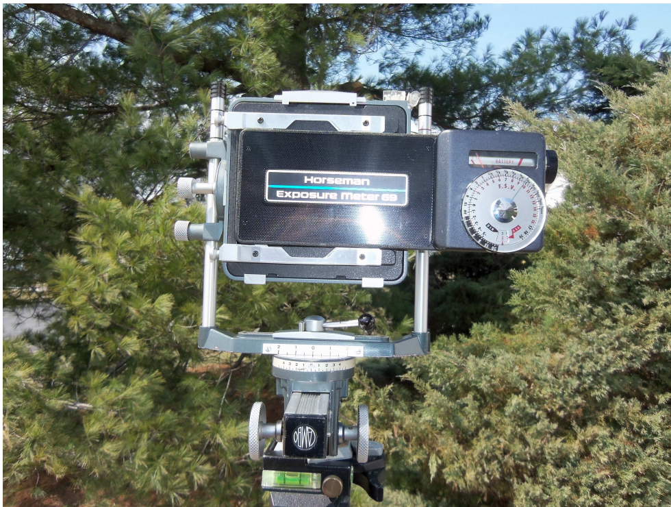
Figure 3: Meter held to 2x3 Cambo back by Graflok sliders
