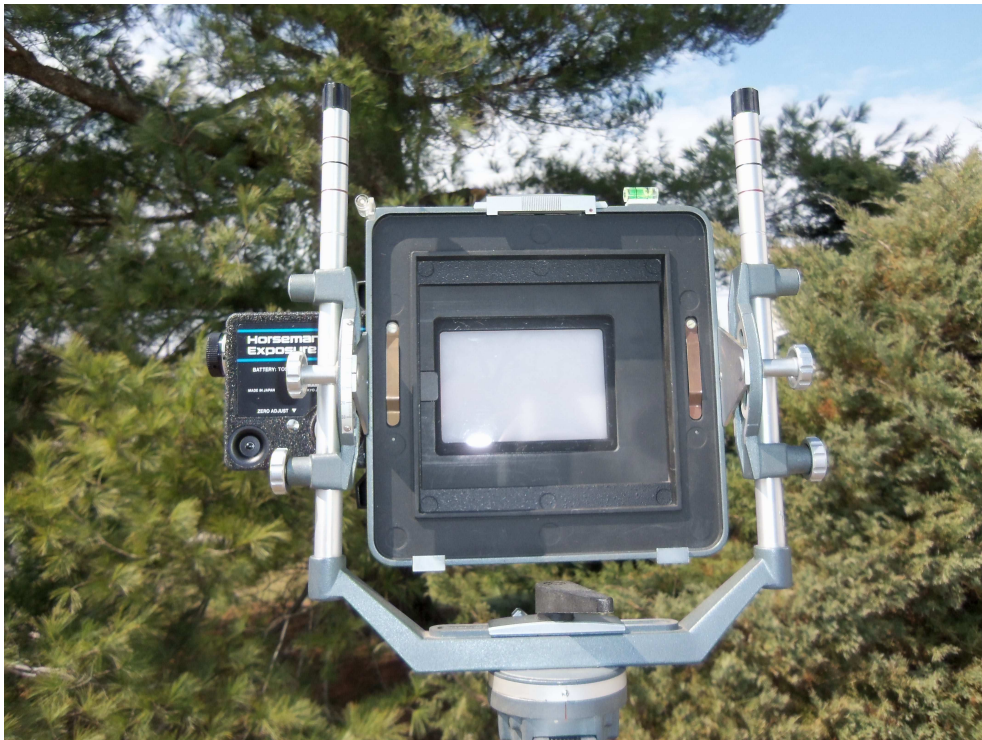
Figure 7: Meter in adapter in 4x5 Cambo back, front view
