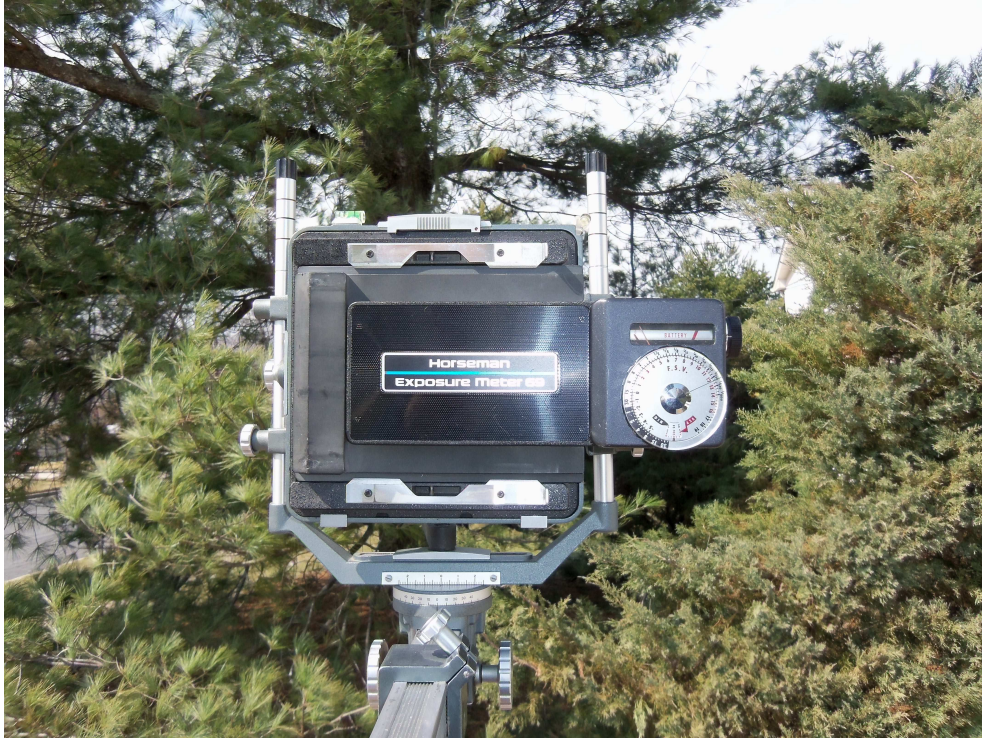
Figure 6: Meter in adapter, held to 4x5 Cambo back by Grafflok sliders
