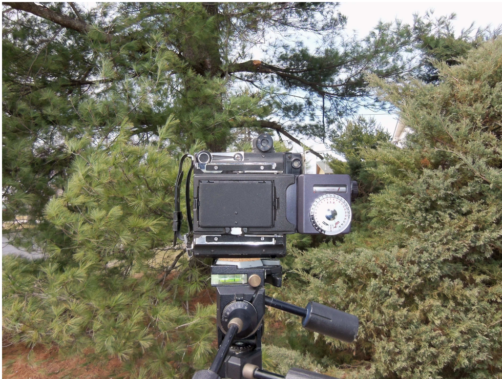
Figure 5: Meter in 2x3 Crown Graphic, held by focusing panel
