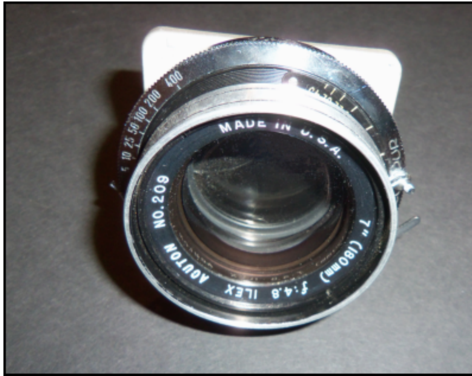
Fig. 2 180/4.8 Acuton in Synchro Compur #1. I bought it as a pair of cells with no shutter. The new Compur's aperture is scaled for the cells combined (180/4.8) but not for a single cell.
