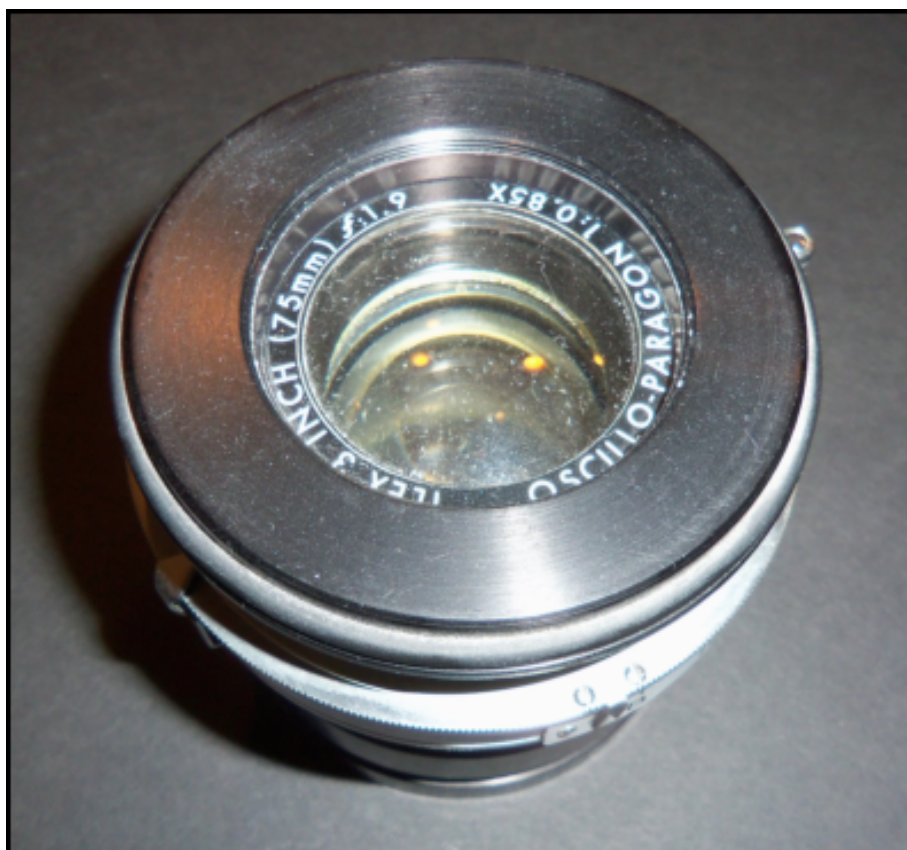
Fig. 1 75/1.9 Oscillo Paragon in #3 Ilex Universal. This lens is dusty because I don't use it. It is, for my purposes at least, completely unusable. I bought it for the shutter.
