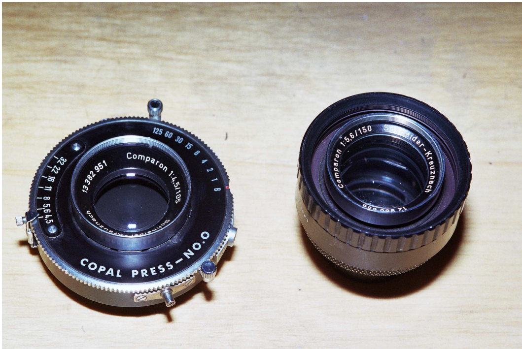
Figure 7: Two Comparons: Schneider's Comparons are essentially Xenars optimized for relatively small enlargements, perform very well as macro lenses. Cheap and cheerful.
