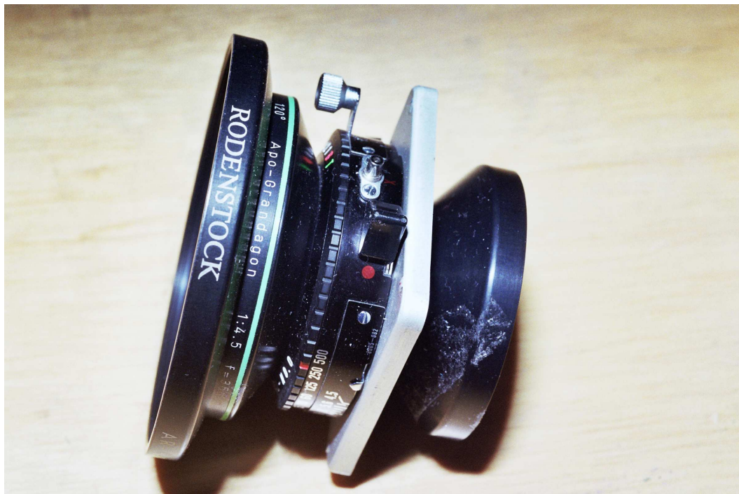
Figure 8: The shortest lens that covers 2x3: So far, the 35/4.5 Apo Grandagon is the shortest commercially available lens that covers 2x3. Its only competitor is the 38/5.6 Super Angulon XL.
