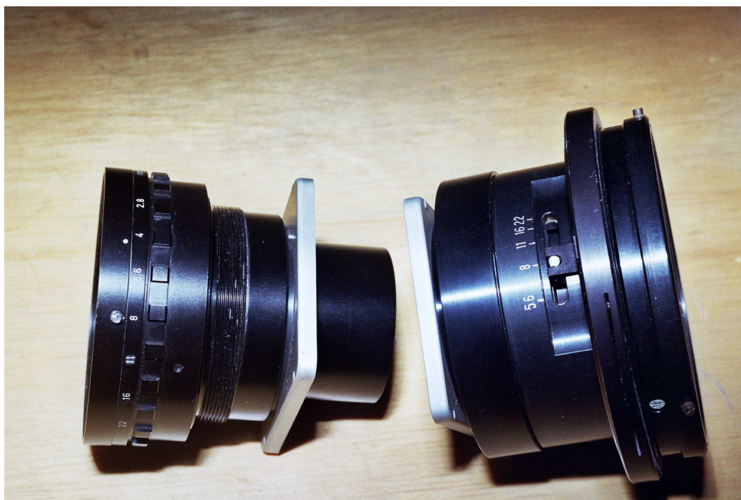
Figure 11: Wide angle aerial lenses on their boards: The Elcan is a retrofocus lens, can be used on a 2x3 Speed Graphic because of that and its mechanical design. The S.F.O.M. is of "normal" construction, neither retrofocus nor telephoto, and just makes infinity on a 2x3 Speed Graphic.
