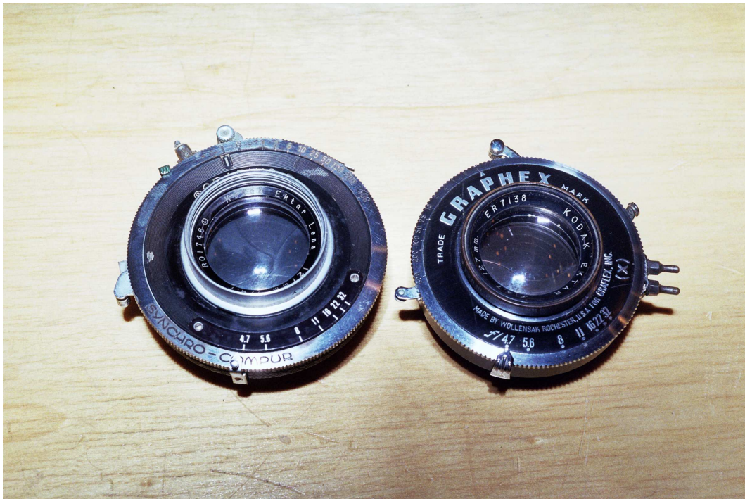
Figure 36: Classic lens, classic shutters: The 127/4.7 Ektar was made to fit Supermatic and Graphex (= Rapax) shutters, both US-made, and the #1 Compur. Kodak, who made Supermatics, and Wollensak, who made Rapaxes (= Graphexes), never agreed on shutter dimensions and both disagreed with Deckel. All three types of shutter work well if in good condition.
