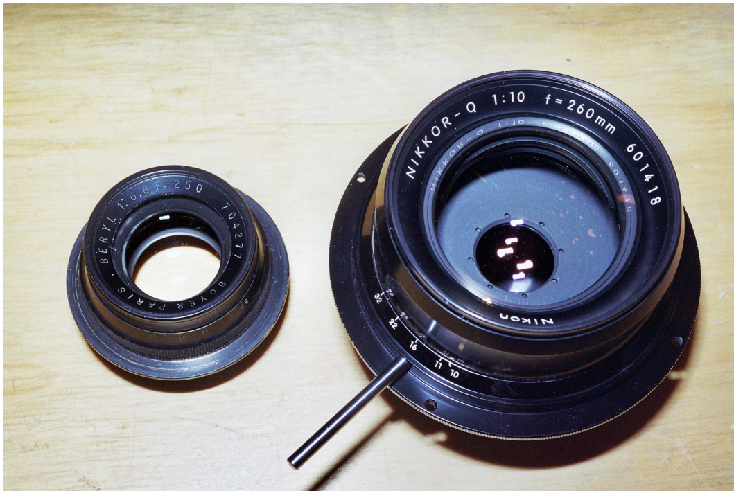
Figure 47: Ten inches: My 260/10 Nikkor-Q's focal length is, according to the quality control sheet, 266 mm. It is identical to the lens later sold as Process Nikkor. For more information on it, see http://homepage2.nifty.com/akiyanroom/redbook-e/ [19], where it is characterized as "Supernatural Grand Lens."
