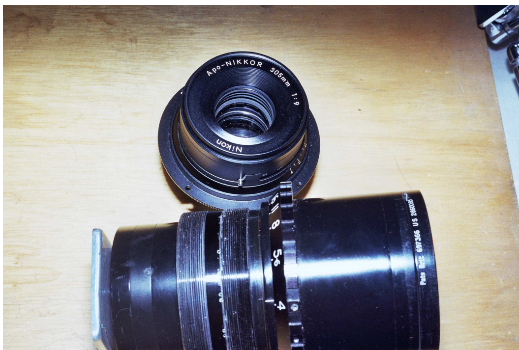
Figure 48: Foot long hot dogs: 305/9 Apo Nikkor, 12"/4 Taylor Hobson Telephoto from an AGI F-139. The 12" tele is much more comfortable fit on a 2x3 Speed Graphic than the Apo Nikkor.
