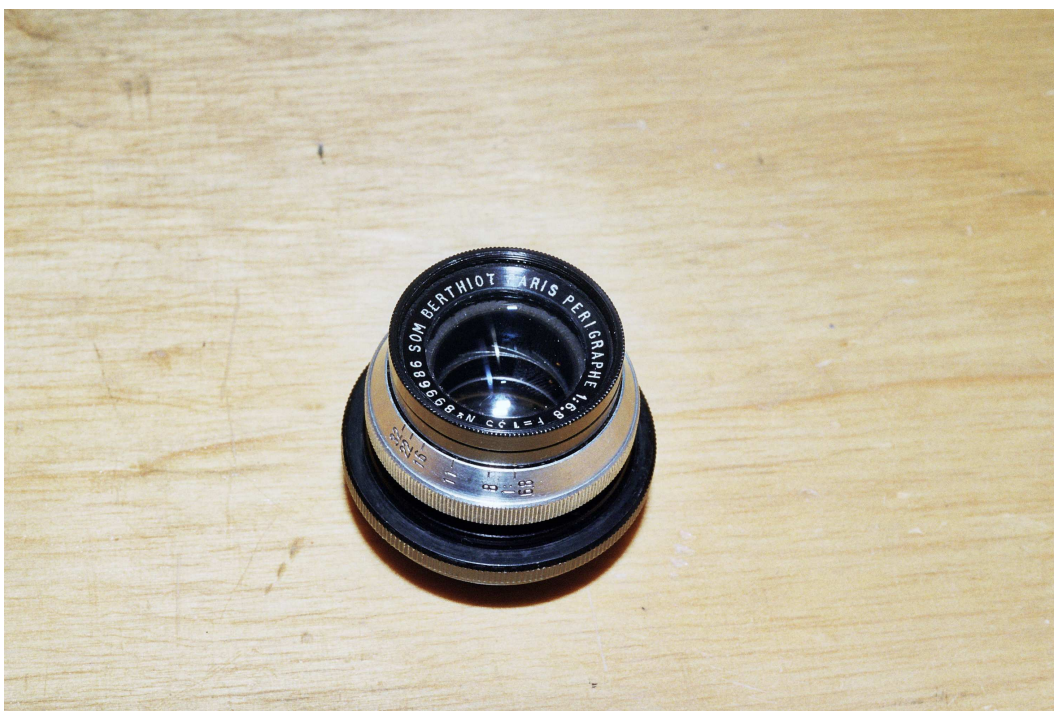
Figure 38: Fast (they say) Périgraphe. In 1912 the f/6.8 Périgraphe was advertised as “Extra-Rapide.” Our concept of “fast lens” has changed a little since then . . .
