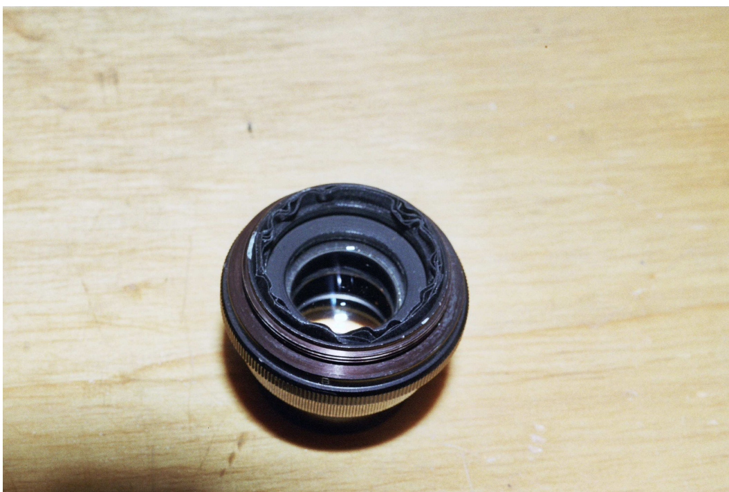
Figure 39: Another way to attach a lens to a Leica extension tube. My little 135/6.8 Périgraphe will fit inside a Leica extension tube that in turn fits an M39x26 tpi-to-#1 adapter. To make the lens stay put I wrapped its threads with darkroom tape. Looks untidy, works.
