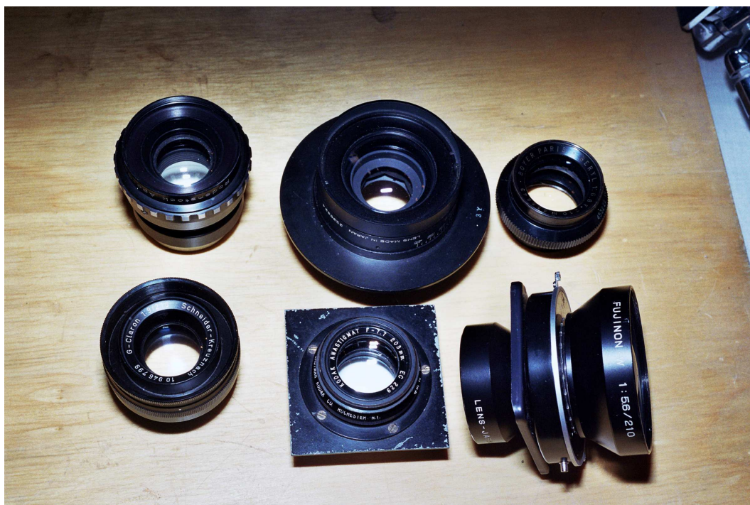
Figure 46: Eight inches: Upper left is a 210/5.6 Apo Gerogon, upper center is a 210/9 Konica Hexanon GR II, and upper right is a 210/6.8 Beryl. If I had to pick one, I'd use the Beryl. But in fact I use a 210/7.7 Beryl S, not shown here.
