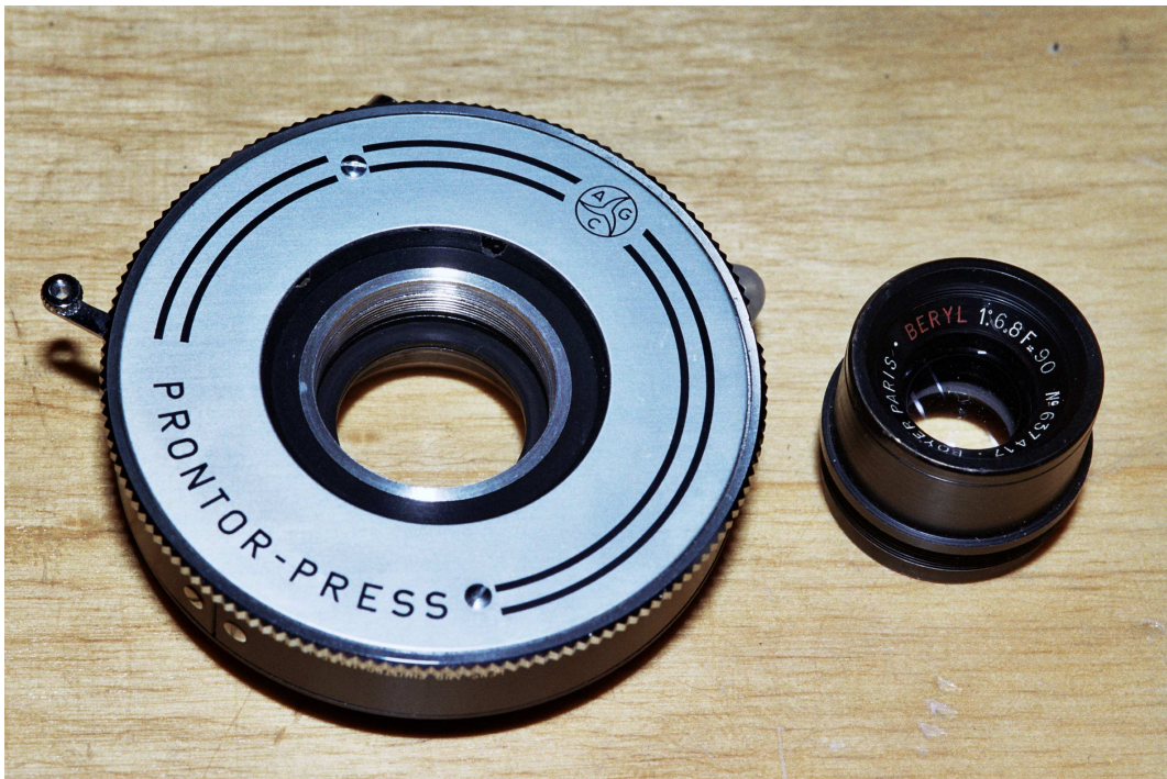
Figure 20: Latest acquisition and its new home: That 90/6.8 Boyer Béryl was extracted from a Chevet Wild Endoscopographe. It is in a plain barrel, so can be used only at full aperture. The cells, however, go directly into a #00 shutter. Before I can use the lens I'll have to have the shutter's aperture scaled for it.
