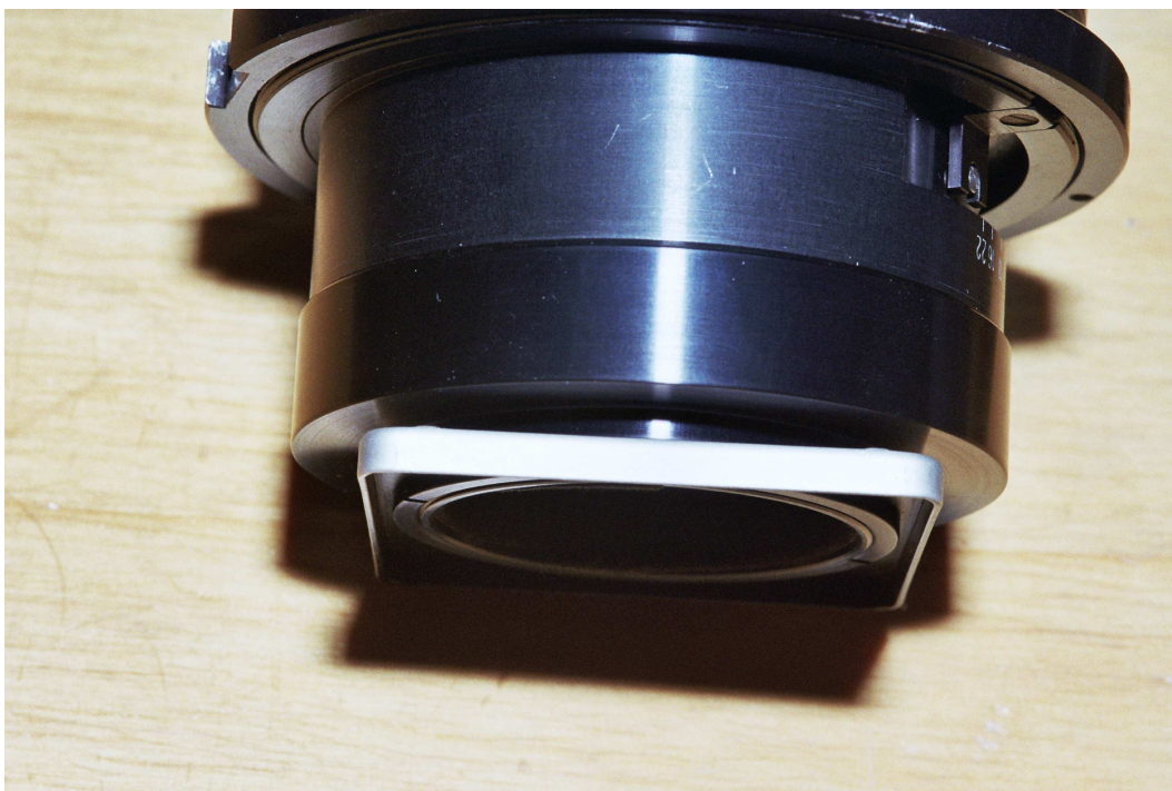
Figure 25: 100/5.6 S.F.O.M. mount adapter: the lens screws into a stepped cup-shaped adapter that is held to the lens board by a normal retaining ring
