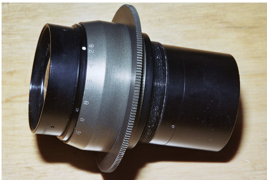
Figure 41: You can have her: The Too Fat Polka (lyrics, in English, at http://lyricsplayground.com/alpha/songs/t/toofatpolka.shtml [17]) describes this lens well. Its back focus is so short that it won't focus to infinity mounted on a 2x3 Graphic board, it won't pass through a 2x3 Graphic's front standard, and, alas, it covers only 6x6.
