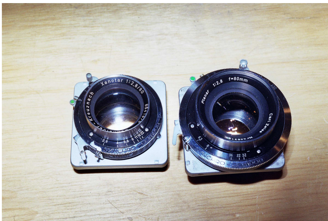
Figure 16: Two answers to the same question: fast normal lenses for 6x6 from Schneider and Zeiss.
