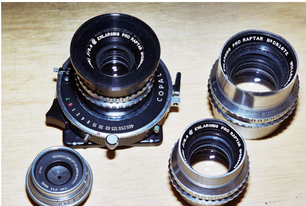
Figure 4: US-made lenses good for macro: Pro Raptars were 6/4 plasmat [10] types and were Wollensak's answer to, e.g., Sironar and plasmat type Symmar taking lenses. Enlarging Pro Raptars were Wollensak's answer to Componon and Rodagon enlarging lenses, were made in focal lengths from 50 mm to 190 mm. The 4"/5.6 Enlarging Pro Raptar, show front-mounted on a Copal #1 shutter, is competitive with the 100/6.3 Luminar for magnifications from 1:8 to 4:1.
