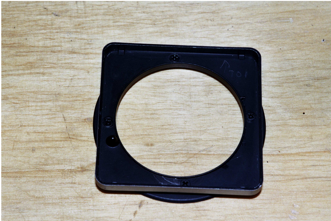
Figure 23: Uran-27 mount adapter rear: the adapter is held to the lens board by four screws, screws into the back of the lens
