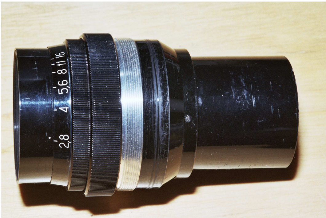
Figure 33: Era-7b: its mounting threads are very far forwards and its rear won't pass through a 2x3 Graphic's front standard. A cup-shaped mount adapter can be made for it but would be very expensive.
