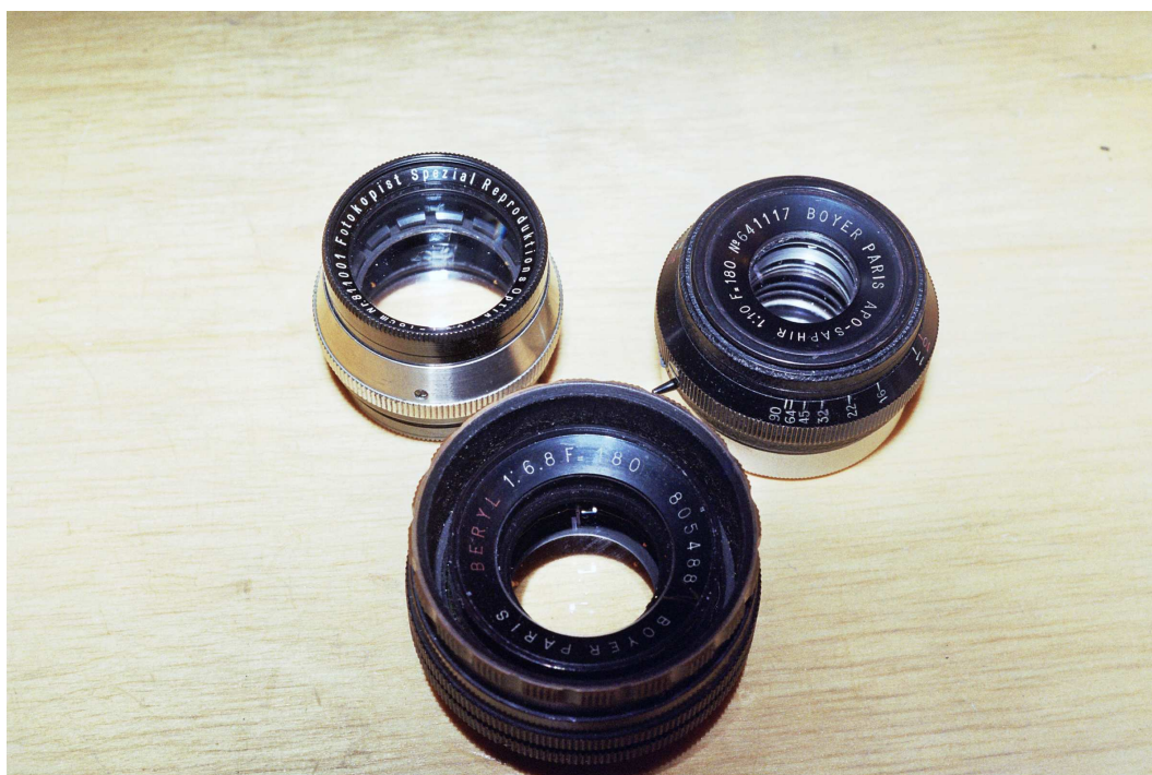
Figure 45: Seven inches: The Apo-Saphir is best, the Fotokopist the worst – I regard it as unusable for general photography – but the Beryl is the best compromise for 2x3.
