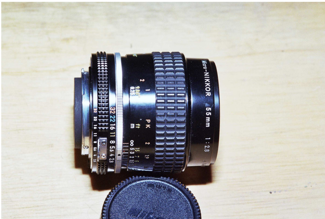
Figure 5: Outstanding macro lens: The 55/2.8 MicroNikkor AIS is a superb lens and can be used, reversed, for photomacrography on formats larger than 24x36. It is at least the equal of the 63/4.5 Luminar and much less expensive.
