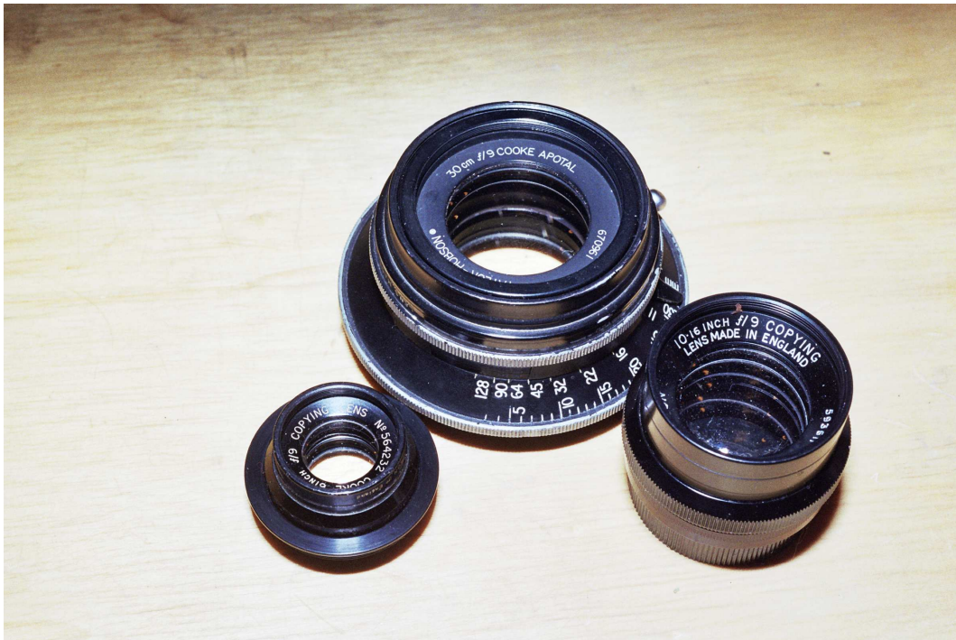
Figure 42: Taylor Hobson tessar type process lenses: different mechanical designs, apparently the same prescription. All are superb.
