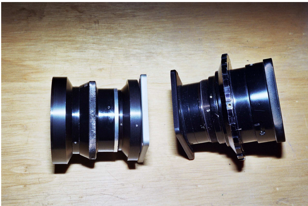
Figure 24: Fast normal lenses on their boards: Lenses too fat to pass through a 2x3 Graphic's front standard must be mounted entirely in front of the lens board. The Uran-27 stands out a little - no more than necessary - to allow room for the sliders that hold the board to the front standard.
