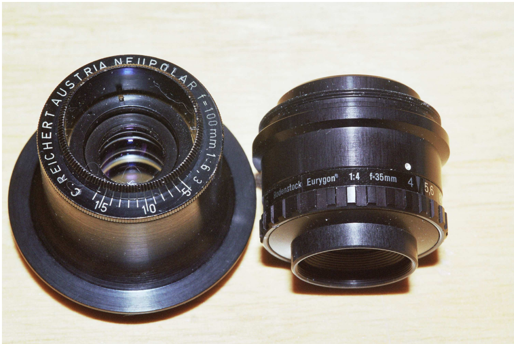
Figure 6: Great and bad macro lenses: the 100/6.3 Neupolar is in an adapter to #1 shutter made by Steve Grimes. The 35/4 Eurygon will screw into the front of a #1.
