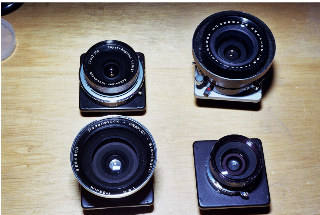
Figure 13: More wide angle lenses for 2x3: 47/5.6 Super Angulon, 58/5.6 Grandagon, 60/5.6 Hexanon, and 65/8 Ilex. All very usable.
