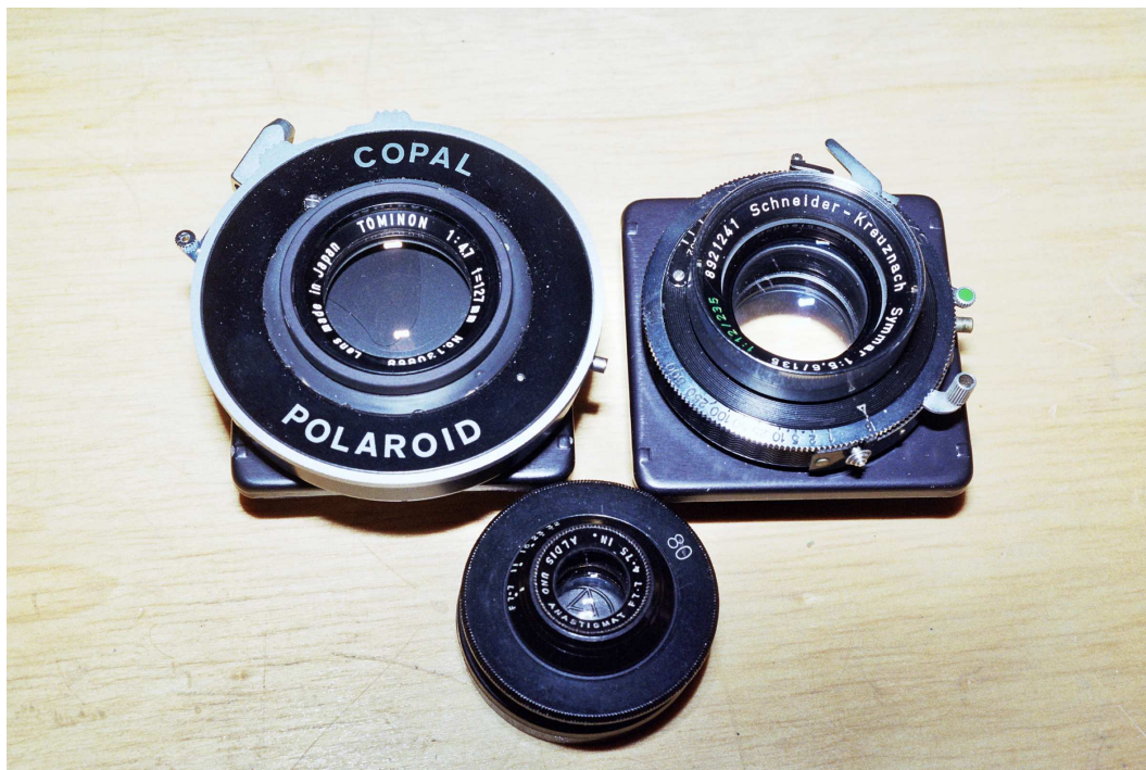
Figure 35: Five inches or so: Three lenses with focal lengths around 5". All are usable, on 2x3 the 127/4.7 Tominon seems to be the best.
