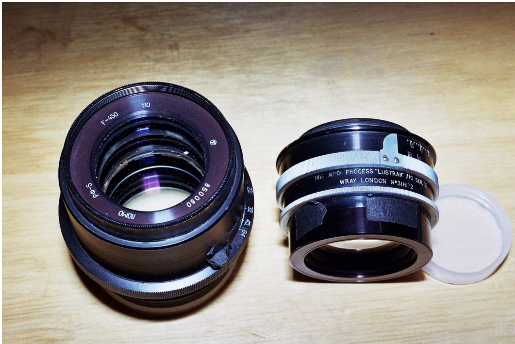
Figure 51: One good, one bad, neither in use: My 450/10 LOMO RF-5 is usable, my 14"/10 Apo Process Lustrar Ser. II isn't; soft below f/22 and flary. I don't use the RF-5 because its focal length is too close to 480 mm.
