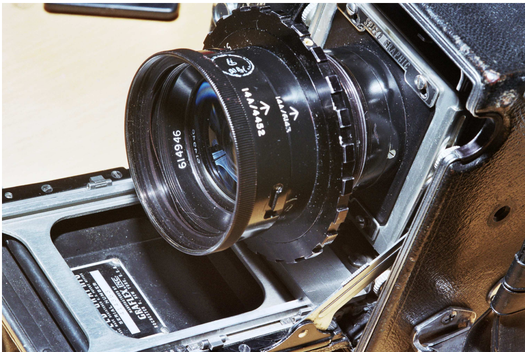
Figure 30: Mr. Lustig's spacer, intended use: the spacer was made to allow the rangefinder to be calibrated for the 4"/2.0 Taylor Hobson Anastigmat
