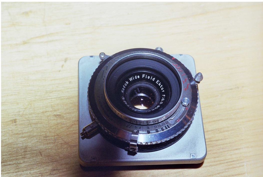
Figure 17: The incomparable 80 mm Wide Field Ektar: The original issue wide angle lens for 2x3 Graphics and a very good lens. Less coverage than, e.g., the similar Cooke Ser. VIIb from TTH and Weitwinkel Aristostigmat from Meyer, but probably sharper.
