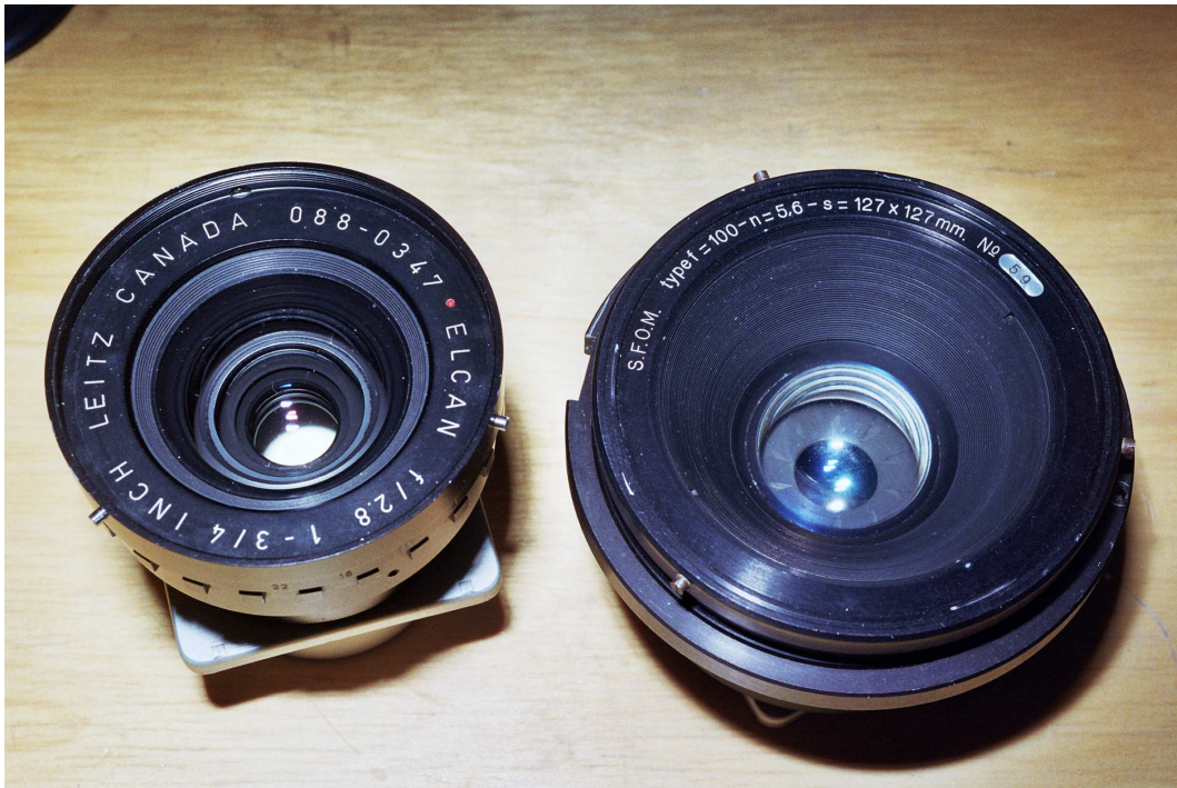
Figure 10: Two ridiculous wide angle aerial lenses: The 1.75"/2.8 Elcan covers 6x6, isn't competitive with the 38/4.5 Biogon, which also covers 6x6, or the 47/5.6 Super Angulon, which covers 2x3. The 100/5.6 S.F.O.M. was made to cover 114 mm x 114 mm on 5" film, is normal, not wide, on 2x3.
