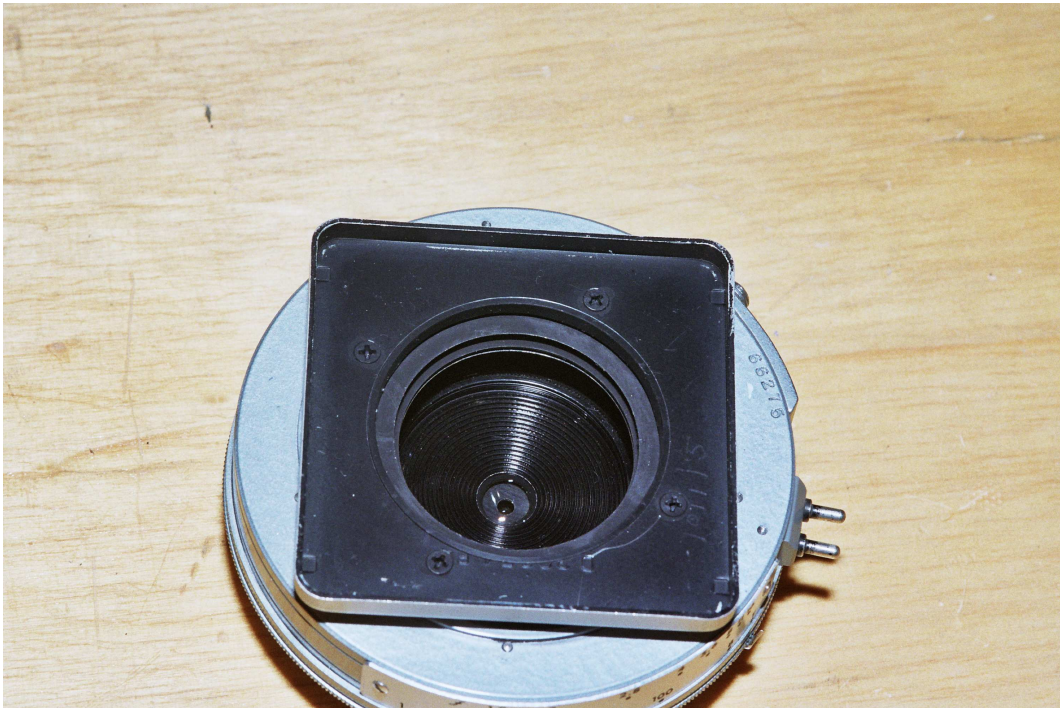
Figure 14: How to attach a mutilated Ilex 3 to a 2x3 Pacemaker board. The shutter's rear tube has been cut off so the usual way of holding a shutter to a board – a retaining ring that screws on to the shutter's rear tube – is impossible. Screws that go through the board and into the shutter do the job.
