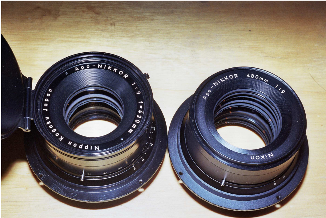
Figure 50: Beautiful long lenses: 420/9 and 480/9 Apo Nikkors. I don't use the 420 because its focal length is too close to 360 mm. On 2x3, both lenses are fully usable wide open.
