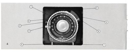
SHUTTER SPEEDS: Shutter Speed Ring (4). Turn until the dot on the raised knurl is opposite the desired speed setting on the shutter speed scale.
